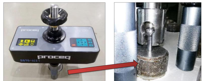
Figure 2. The view of: a) pull-off tests apparatus, b) steel disc glued to the surface
